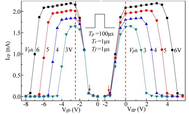
Fig. 3. Elliot curves for HT devices using optimized square pulses ( $T_r = 1 \mu s$  for  $I_{geo}$  elimination) with different  $V_{ph}$ 's.  $I_{cp}$  is plotted against  $V_{gb}$  in the left and  $V_{gp}$  in the right. All curves are similar to those in MOSFETs. In addition, falling/rising edges and positions of central flat regions coincide.
