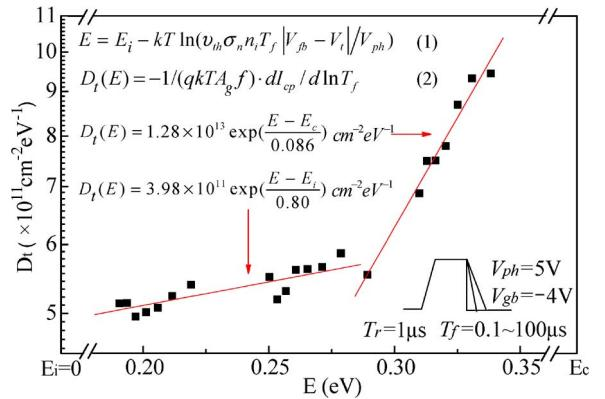
Fig. 4. Typical dual exponential  $D_t(E)$  distribution between the midgap ( $E_i$ ) and the conduction band ( $E_c$ ) for HT devices extracted with (1) and (2) using optimized square pulses.
