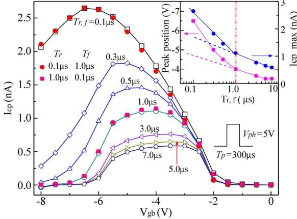
Fig. 2. Elliot curves for HT devices using square pulses with different  $T_r$ 's and  $T_f$ 's. The inset shows the peak position and  $I_{cp\_max}$  (the  $I_{cp}$  values at the corresponding peak positions) that are dependent on  $T_{r,f}$ . At  $T_r > \sim 1 \mu s$ ,  $I_{geo}$  is minimized, and improved CP curves are obtained.
