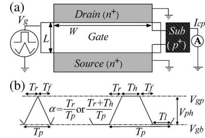
Fig. 1. (a) Device plane view and a schematic diagram of CP measurement. (b) Pulse parameter definition.
