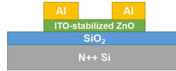
Fig. 1. Schematic of the top-contact bottom-gated TFTs in this work.
