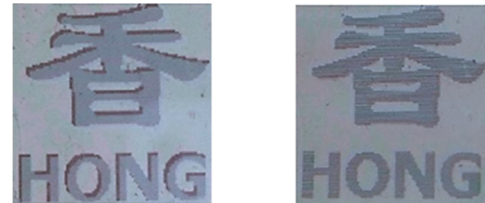
(a) (b) Fig. 6. Two different pictures for different eyes taken from different polarizers on the stereoscopic goggles. [two movies are attached to show the effect for different eye (Media. 1) and the display (Media. 2)]
